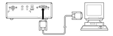
Plug the scanner end of the RS232C straight cable into the remote port which is on the rear of the scanner. Plug the other end of the cable (DB-9 serial connector) into a personal computer's serial port. A few PC's may require an adapter, most will not. Of course, make sure your PC is turned ON.
