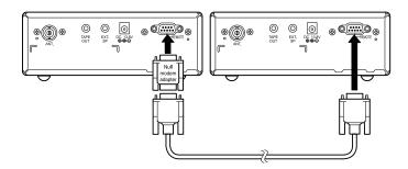
You can clone all of the programming of one UBC785XLT into another, including alpha tags, delay settings, etc. After connecting the two scanners, turn the radios ON. Prepare each scanner for clone mode as follows.
