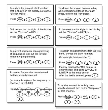
This shortcut card is designed to assist you in getting through the menu screens using the direct entry mode for commonly used features. Please read the manual thoroughly before using this card. Be sure to back out of the menu screen after each shortcut by repeatedly pressing MENU or by pressing SCAN or SRCH keys.
