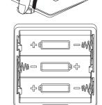
Note that the batteries are intended to provide backup power for the clock and for scanning for a short time. When the backup batteries becomes too low, appears. Promptly replace the batteries.
