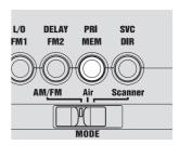
To quickly recall a channel, select the band, select the channel memory mode by pressing **PRI/MEM**, then tap the number button that corresponds to the memory where the channel is stored.
