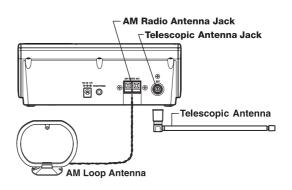
the scanner and twisting it to the desired angle. Connect the two wires from the loop antenna to the **AM RADIO ANT** terminals on the back of the scanner.
